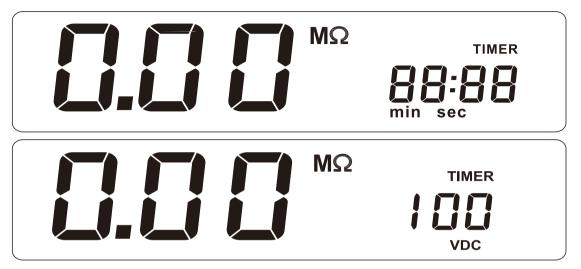
Press SELECT to check the preset time. The LCD screen display TIMER, PRES is shown on primary display, the secondary display shows the preset time. Press ENTER, the meter display Set. The time can be adjusted by  $\triangle/\triangledown$  button. Presws ENTER again to confirm the adjustment.
