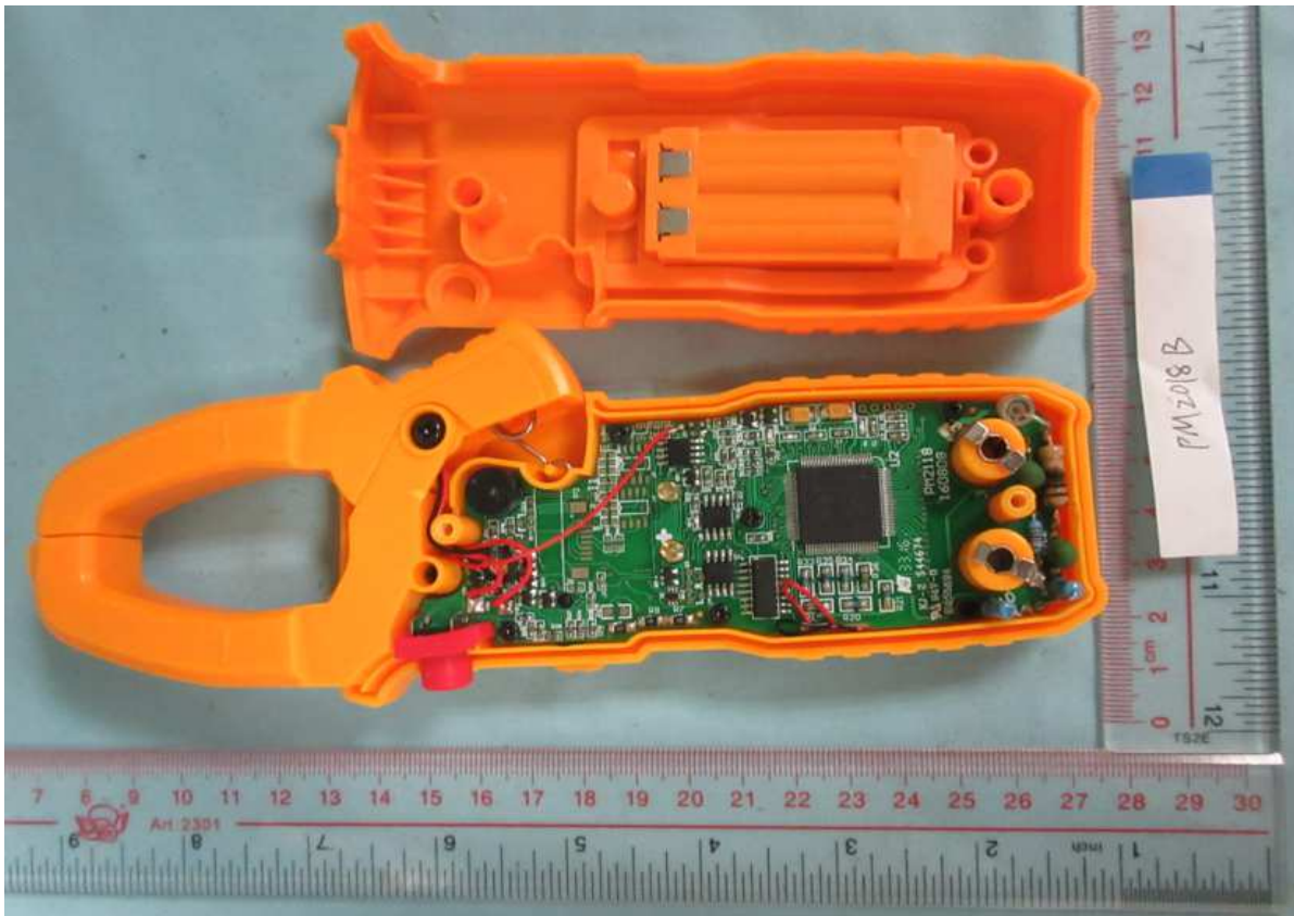
Photo 8: Internal view of PM2018B
