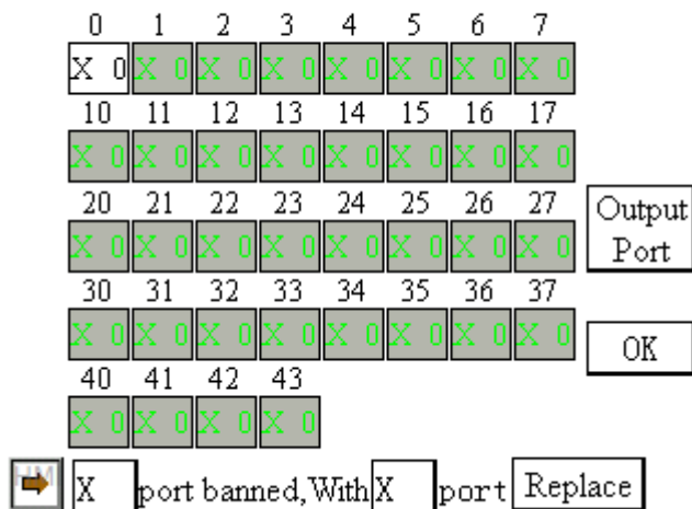
Touchwin HMI I/O terminal exchanging screen
